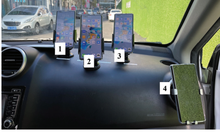
Fig. 4. The installation position of the smartphone in the vehicle. Only the sensor data of one smartphone is used in a single test.
